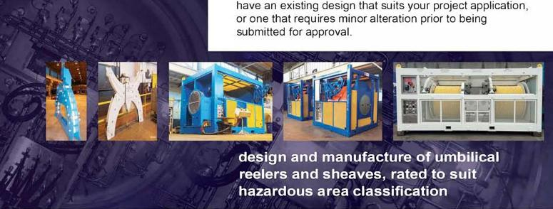
All HCS Control Systems reelers are designed to either DNV 2.7-1 for those units weighing less than 25 Tonnes or DNV 2.7-3 where weight is greater than 25 Tonnes. Units are CE Marked accordingly to suit Hazardous Area Classification.
